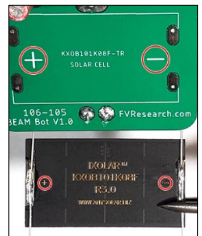
Figure 6 - Match up polarity signs on solar cell and PCB
